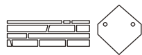
1 Otta murstein 5-25 cm. Otta takskifer 38 x 38 cm (15"). Otta bricks 5-25 cm. Otta roofing 38 x 38 cm (15").
