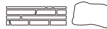
3 Otta murstein 5-25 cm. Bruddhelle som vindusbrett. Otta bricks 5-25 cm. Crazy paving as window sill.
