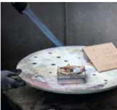
Various products can be mounted onto our plaques. We make sure that the plaque and the modeled item get patinated together to ensure the patinas work with each other.
