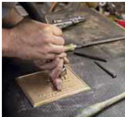
After the sand casting is completed, every plaque is chased by hand to ensure the highest quality and desired detail is achieved.
