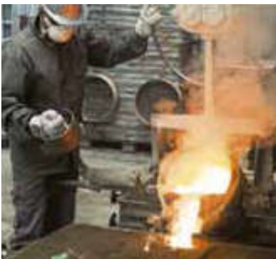
Every Plaque is sand cast. The bronze reaches an approximate temperature of 2282°F.
