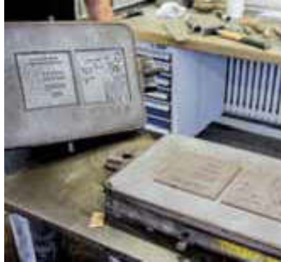
The approved layout is used to create the desired plaque form. From this a positive and negative mold is created.
