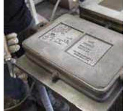
Casting vents are carved into the sand to allow the bronze to flow and take its final form.
